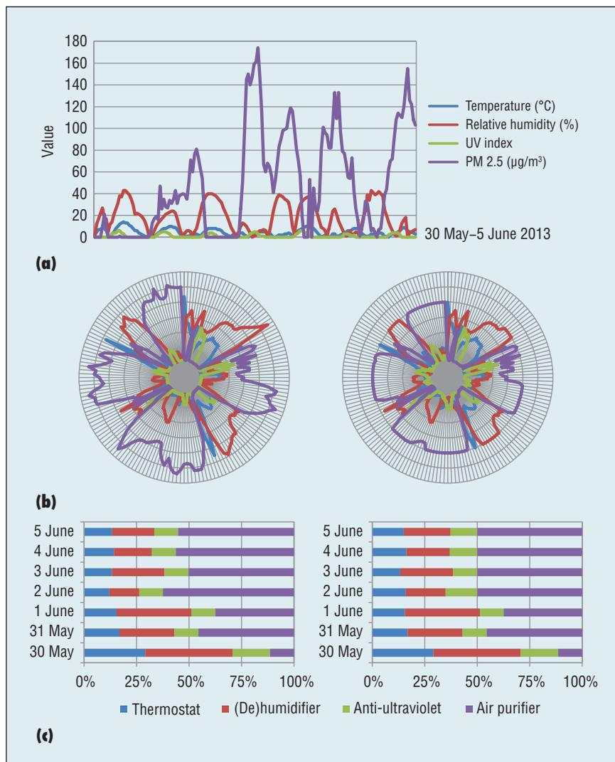
**Figure 4. Data perception and resource allocation. (a) The sensing data during one week according to the defined criterion; (b) the original and revised real-time resource allocation; and (c) the original and revised daily resource allocation, in which  $p = 70$  percent, and the threshold  $T_d = 50$  percent.**
